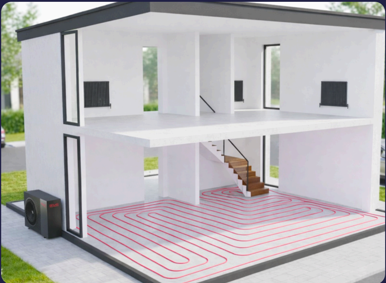
A house using the full Snug ecosystem: underfloor heating, heat pumps, and radiators.
